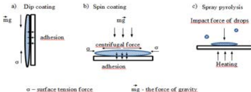
Figure 1 – Scheme of the distribution of forces depending on the deposition technique
