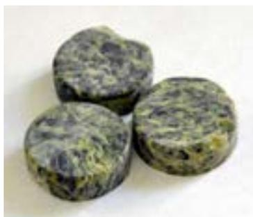
**Figure 1** – Sliced up samples of serpentine drill-core prepared for the investigation
