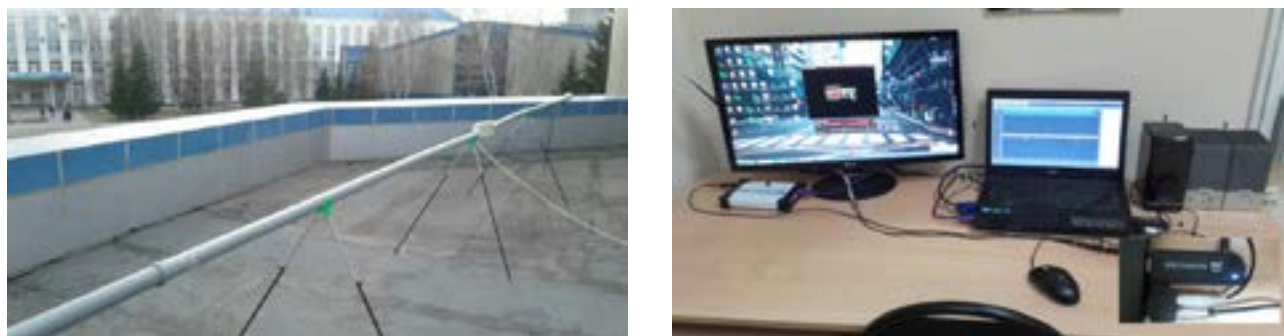
Figure 6 – Antenna (upper part) and an instrument complex for registering meteors in the radio range.
