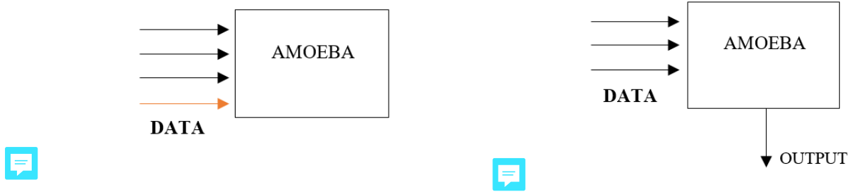
Рис. 11: Learning phase of AMOEBA, with the given oracle (red arrow) Рис. 12: The exploitation step of AMOEBA, without labeled data
