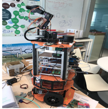
Fig. 2: The picture of the real robot with 4 DOF named TwIRTe
