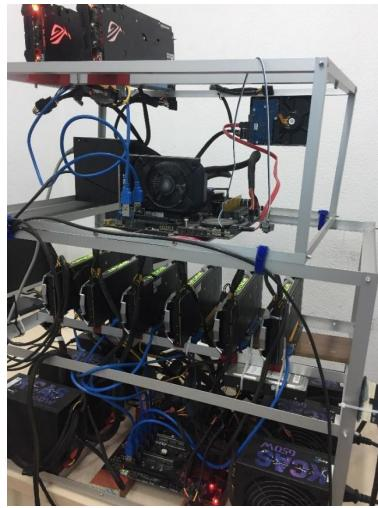
**Figure 3** – Example of cryptocurrency miner setup: at the bottom level Setup #1 is shown; at top Setup #2 is shown. We compare data to the average power consumption of Desktop PC with LCD Display [15].
