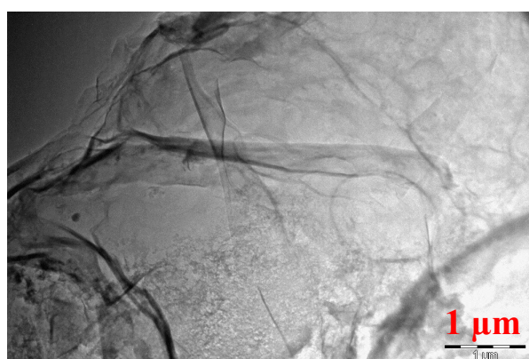
Figure 7 – TEM microimages of the graphene layers
