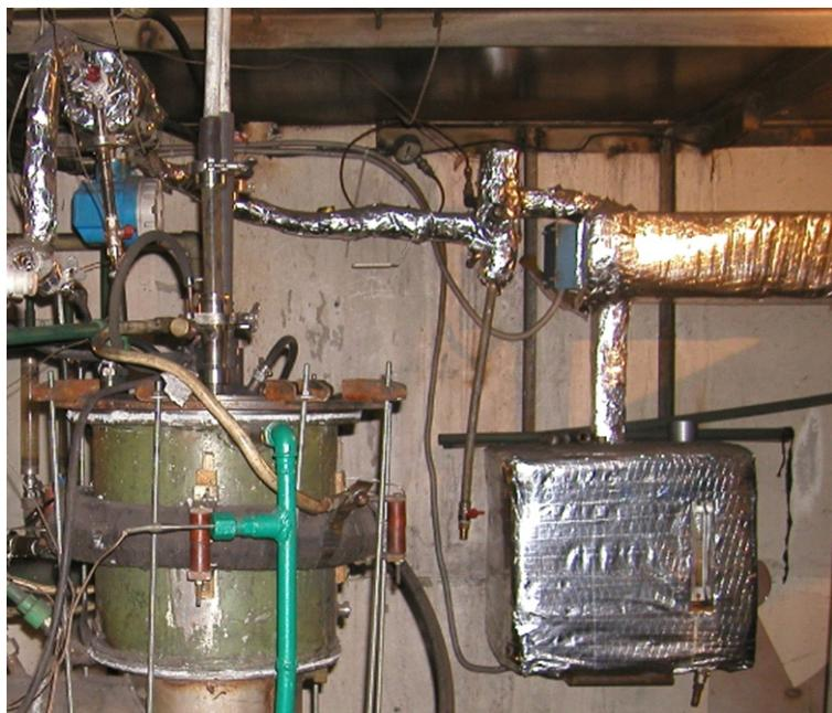
**Figure 7 –** Reactor steam supply system
