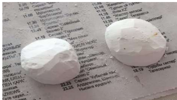
Figure 1 – Limestone (chalk) – model material of a carbonate oil reservoir
