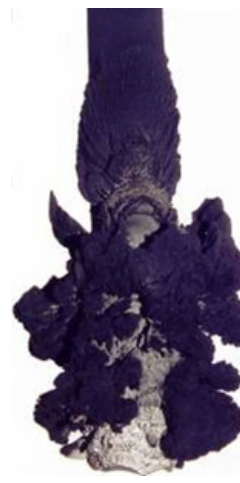
Figure 3 – Appearance of the platinum-containing deposit on the cathode.
