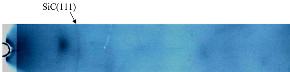
Figure 3 – X-ray diffraction pattern of thin SiC x film deposited by magnetron sputtering, after annealing at 1100°C for 30 min in an Ar atmosphere
