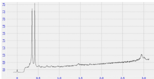
Figure 2 – Raman - spectrum of molybdenum disulfide on a silicon substrate.
